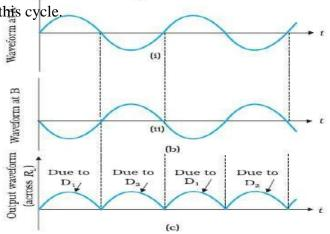
The input waveform (ac source)
